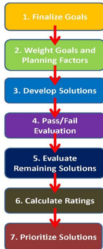
FIGURE 1 Seven-step Process for Solution Evaluation
